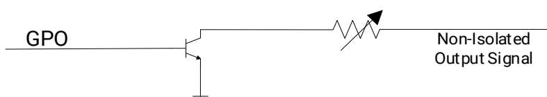
Figure 5-3 Internal Circuit of Output Signal
