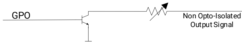
Figure 6-9 Internal Circuit of Output Signal
