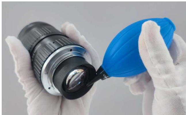
Figure 2-1 Cleaning by Rubber Dust Air Blower
