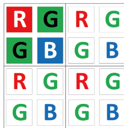
Figure 11-11 Horizontal/Vertical Binning 2 × 2 (Color Device as an Example)
